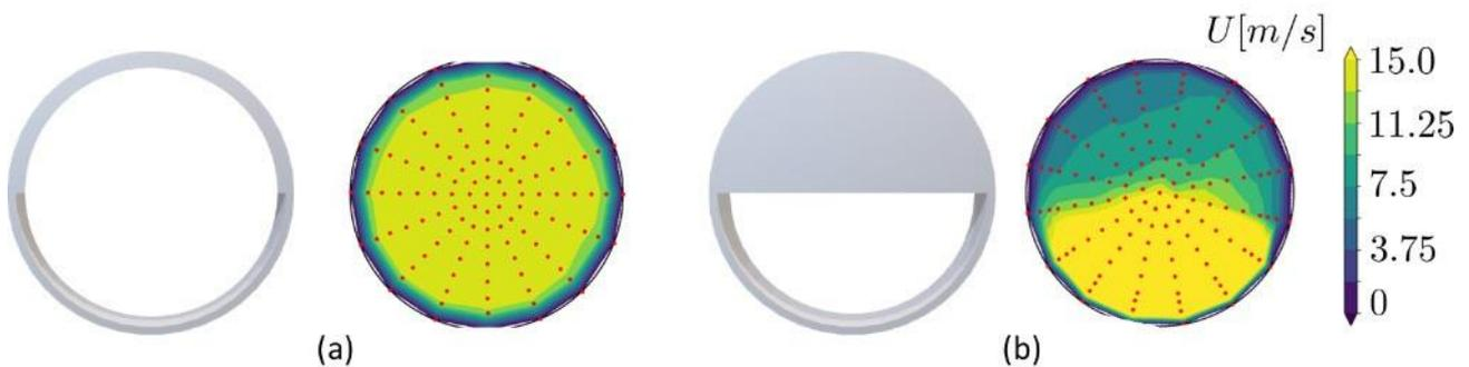
Figure 2: Distortion grids and respective axial velocity map at 50 mm from the fan inlet.
