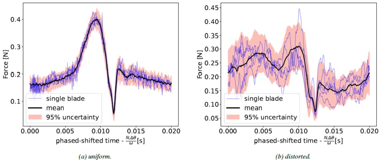
Figure 6: phased-locked time signal of the blades loading's under (a) uniform inflow and (b) distorted inflow
