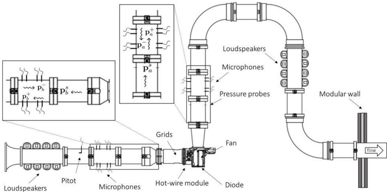
Figure 1: An illustration of the instrumentation of the facility. The vectors  $\mathbf{p}^+$  and  $\mathbf{p}^-$  are respectively the incident and outgoing acoustic pressure fluctuations in each mode. The vector  $\mathbf{p}_s$  is the source vector. The indices  $a$  and  $b$  shows the downstream and upstream side of the multi-ports
