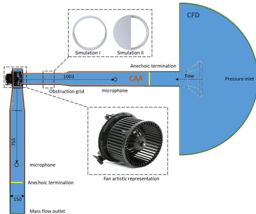
Figure 4: Schematic geometry of the fan and test facility regions. The CFD region used for the LES turbulent flow simulation is highlighted in blue while the Region for the sound propagation is shown in red with all dimensions in mm.
