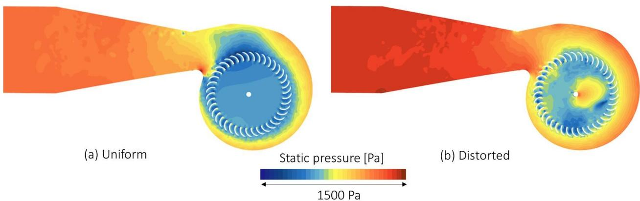
Figure 7: Static pressure distribution in a plane perpendicular to the wheel at 50 % of span in (a) uniform (b) distorted inflow.
