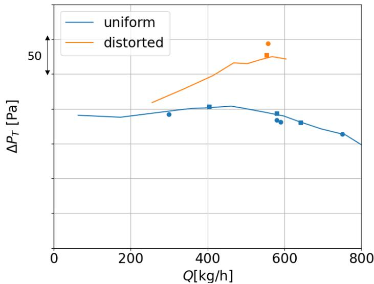
Figure 5: Total pressure performances curves under uniform and distorted inflow. The experimental measurements —, acoustic multi-ports measurements □, URANS simulations •.
