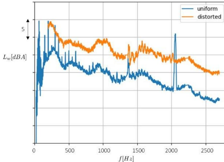
Figure 3: Comparison of the fan noise emission downstream of the fan with uniform and distorted inflow at a mass flowrate  $q \approx 580$  kg/h.
