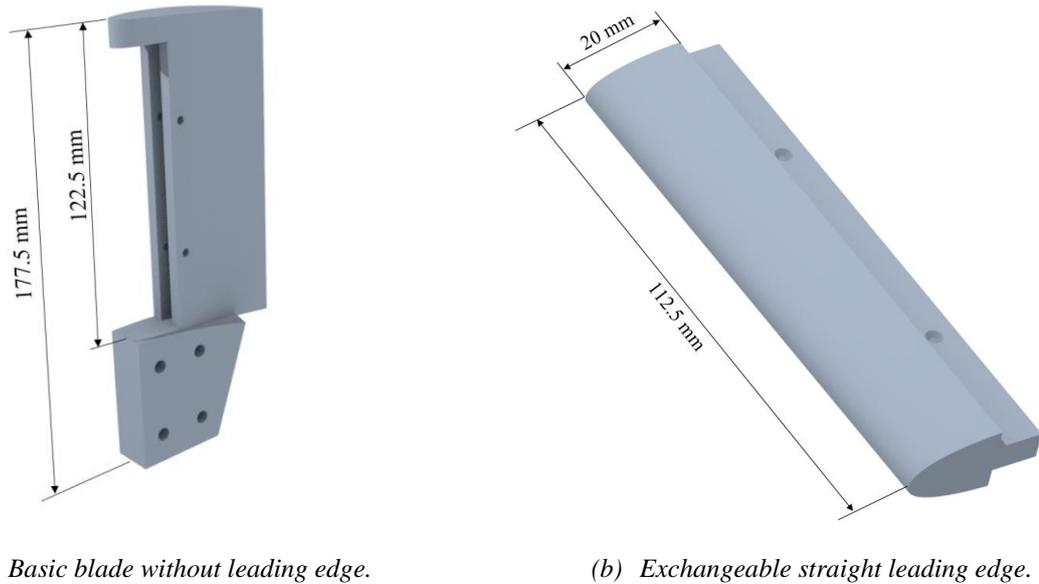
Figure 1: Illustration of the basic blade and a replaceable leading edge. The two components can be connected via a groove and two flat-head screws. In order to provide additional radial securing, the tip area of the blade is designed to be solid.
