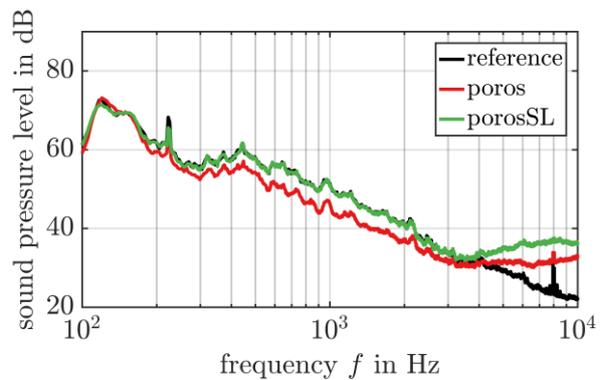
(b) Sound pressure spectra ( $\dot{V} = 1.1 \text{ m}^3/\text{s}$ ).
