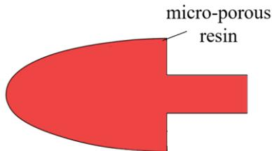
(e) Leading edge made of micro-porous resin.
