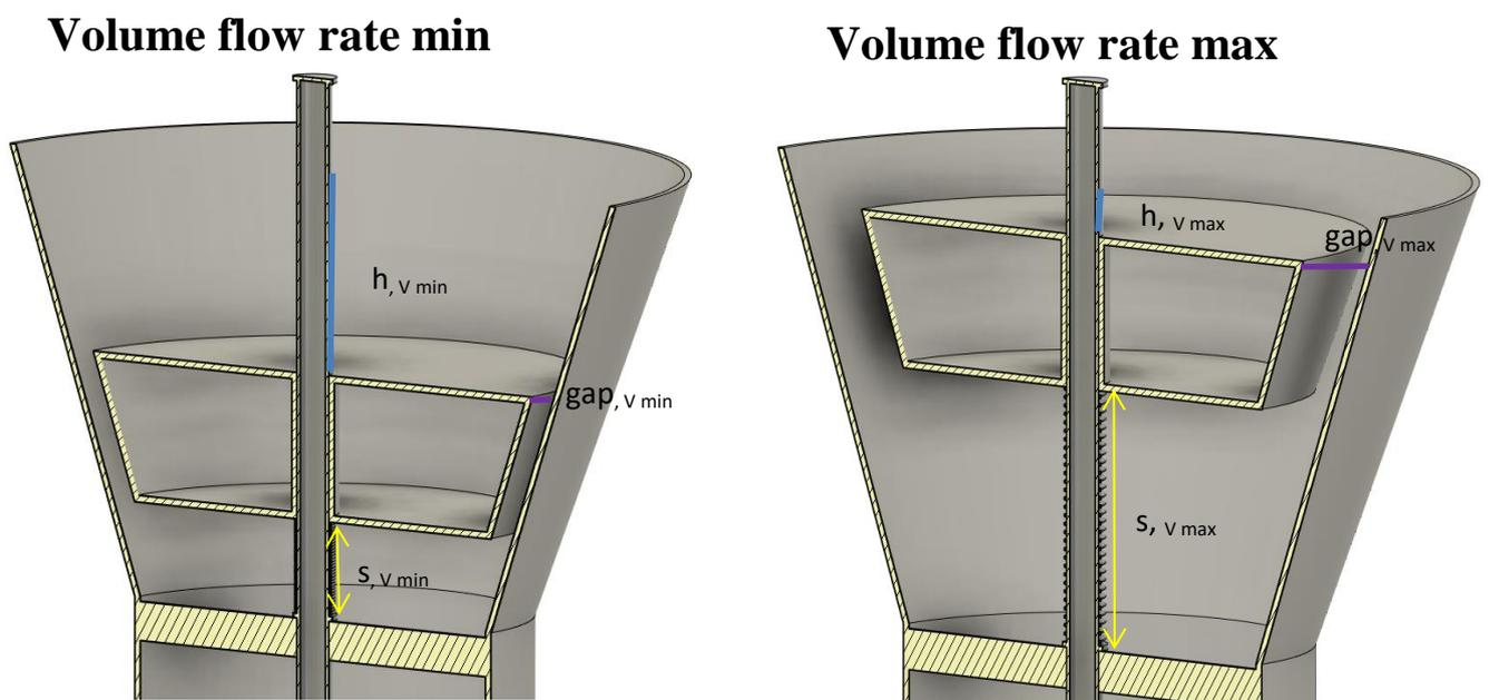
Figure 4: Different heights at different volume flow rates [2]
