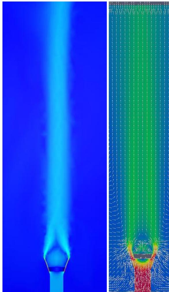
Figure 10: velocity field [m/s] plotted w/o (left) and with speed arrows (right), both sides at:  $\dot{V}_{max} = 1,000 \text{ m}^3/\text{h}$
