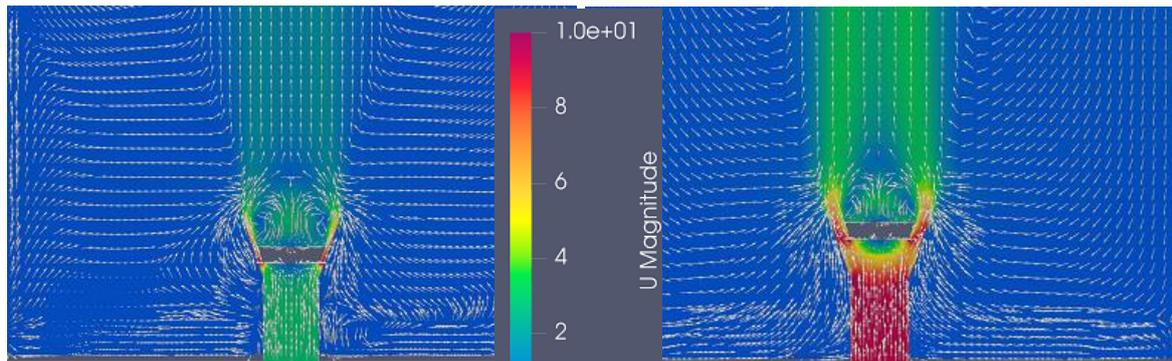
Figure 9: velocity field [m/s] plotted with speed arrows, left side:  $\dot{V}_{min} = 300 \text{ m}^3/\text{h}$ , right side:  $\dot{V}_{max} = 1,000 \text{ m}^3/\text{h}$
