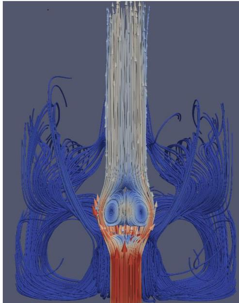
Figure 11: stream function [m<sup>2</sup>/s] plotted with speed arrows at  $\dot{V}_{max} = 1,000 \text{ m}^3/\text{h}$
