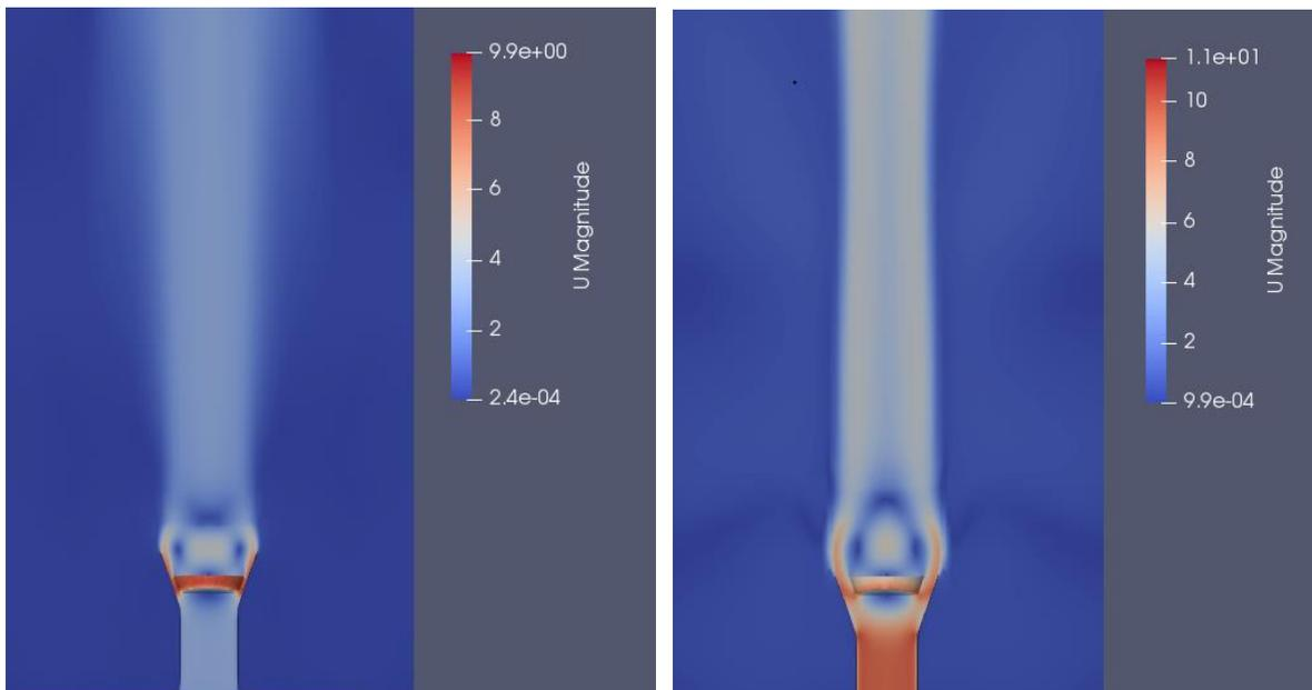
Figure 7: velocity field [m/s] plotted by Paraview [5], left side:  $\dot{V}_{min} = 300 \text{ m}^3/\text{h}$ , right side:  $\dot{V}_{max} = 1,000 \text{ m}^3/\text{h}$
