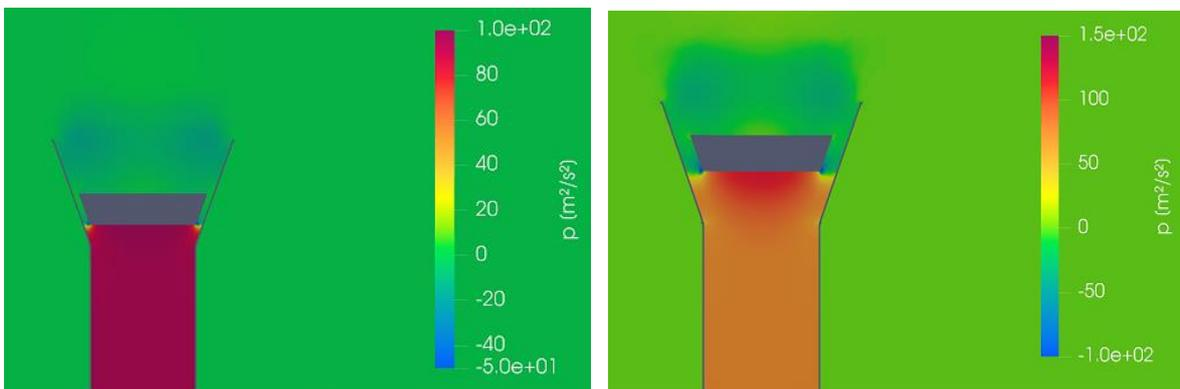
Figure 8: pressure field [m<sup>2</sup>/s<sup>2</sup>] (\* density 1.2 kg/m<sup>3</sup>), left side:  $\dot{V}_{min} = 300 \text{ m}^3/\text{h}$ , right side:  $\dot{V}_{max} = 1,000 \text{ m}^3/\text{h}$
