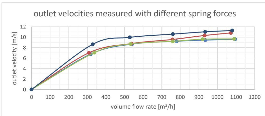
Figure 12: EARC outlet velocities measured with different spring forces at variable volume flow rates size DN200
