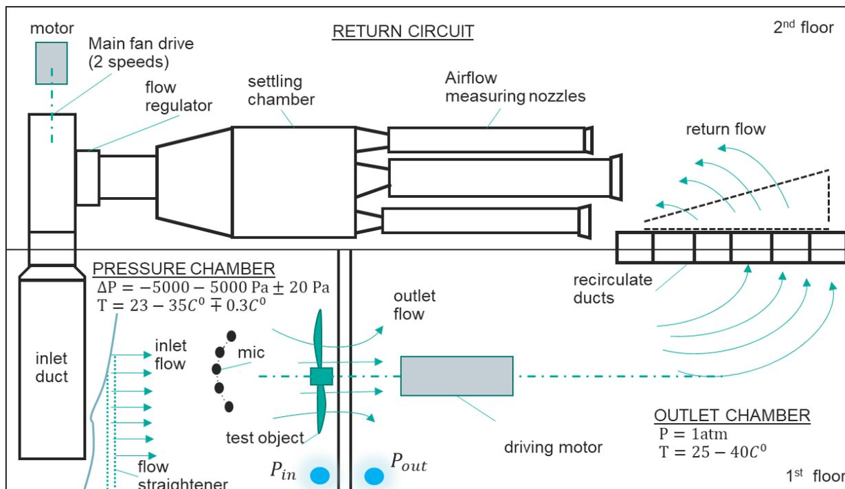
Figure 1: Schematic of fan test rig
