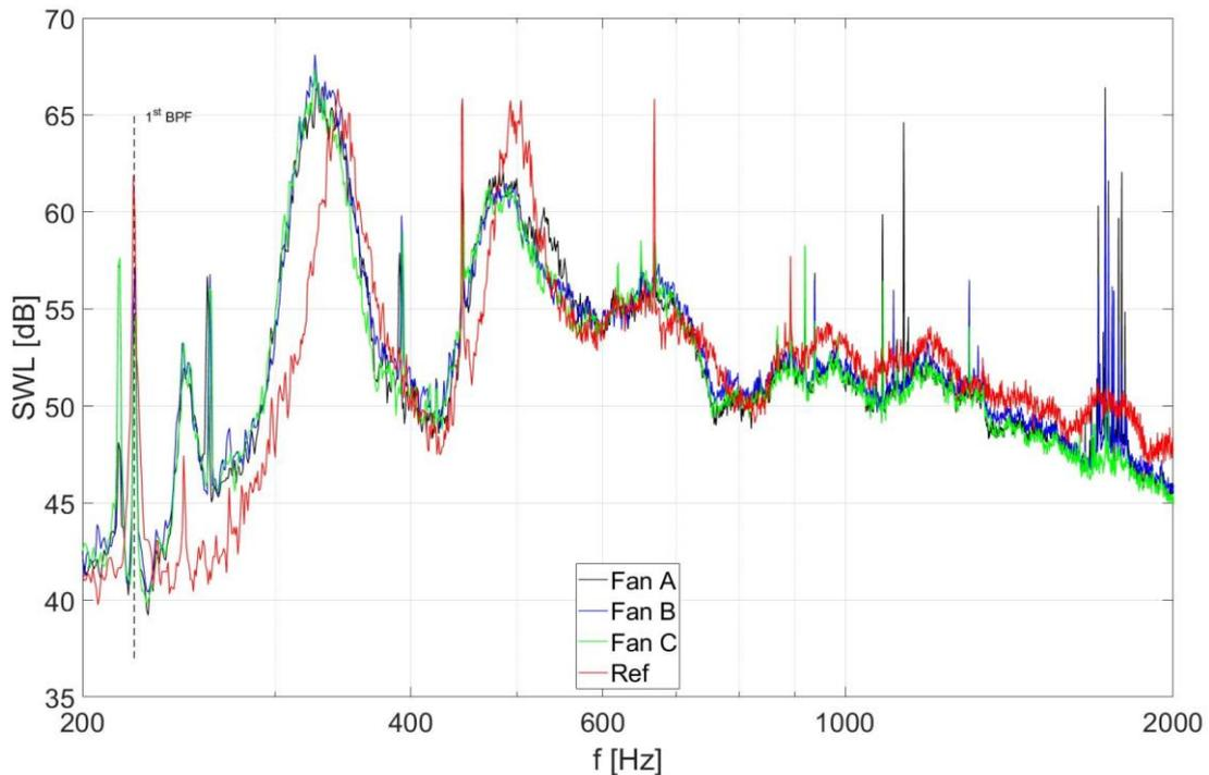
Figure 6: Sound power spectra of 3D printed fans and reference at 1486 rpm, 1.4 m<sup>3</sup>/s
