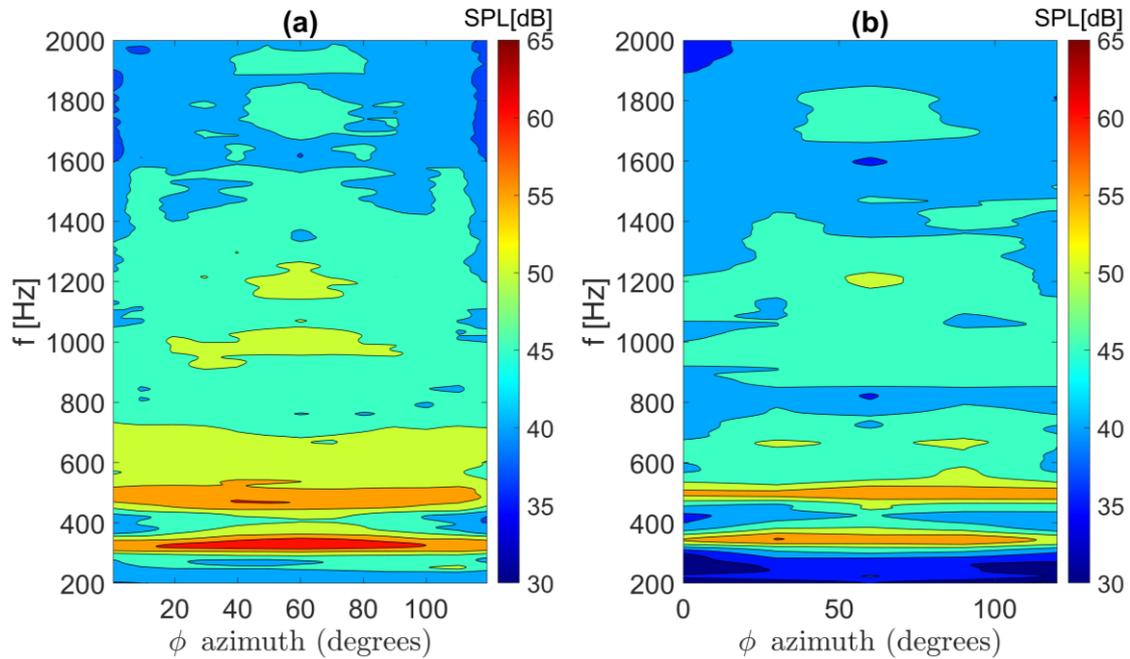
Figure 7: SPL distribution over azimuth angle and frequency at  $0^\circ$  polar angle;
