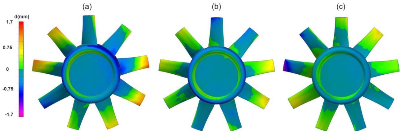
Figure 3: Deviation ( $d$ ) of 3D printed fans from CAD model;
