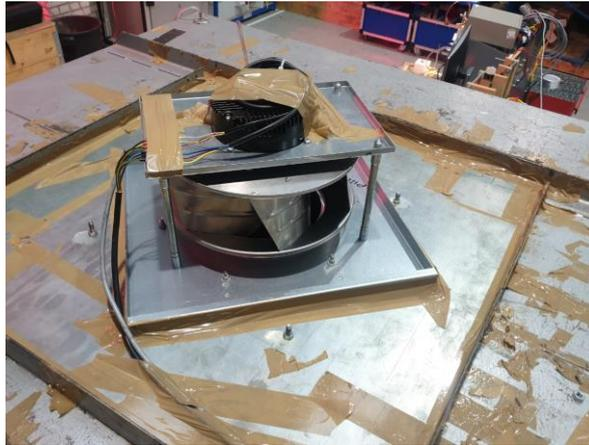
Figure 7: Experimental test setup using plenum chamber
