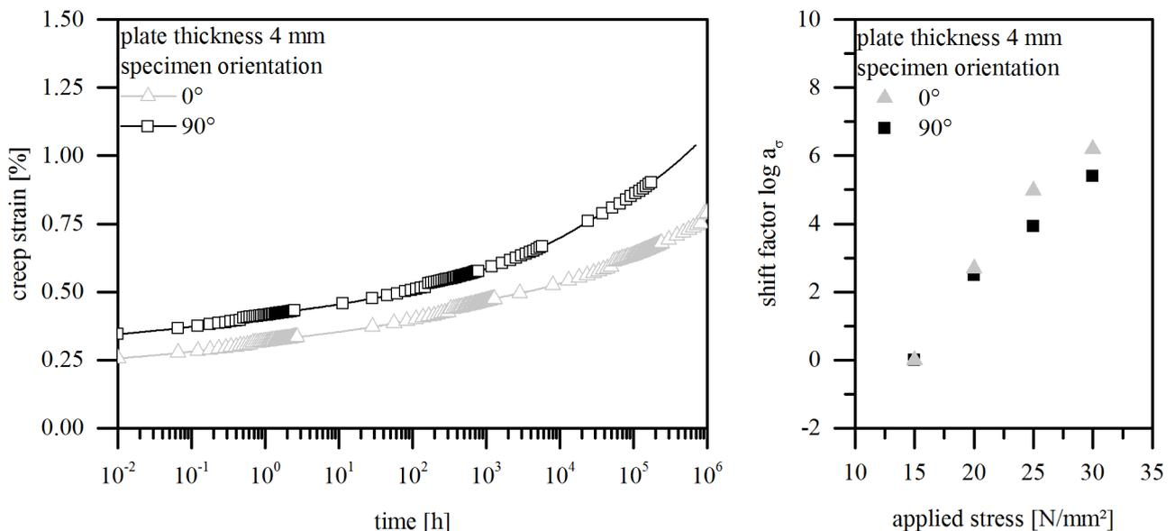
Figure 10: creep master curve for stress of 15 N/mm<sup>2</sup> (left) and shift factor vs. stress (right)
