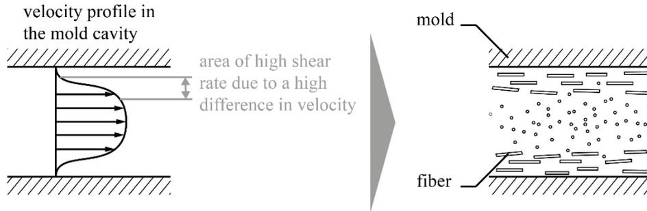
Figure 1: fiber orientation in injection molding due to the shear rate in polymer flow
