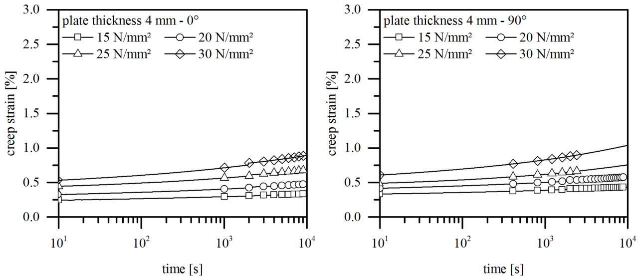
Figure 9: short creep strain curves for with constant stress 15 N/mm<sup>2</sup>, 20 N/mm<sup>2</sup>, 25 N/mm<sup>2</sup> and 30 N/mm<sup>2</sup> for specimen orientations of 0° (left) and 90° (right);
