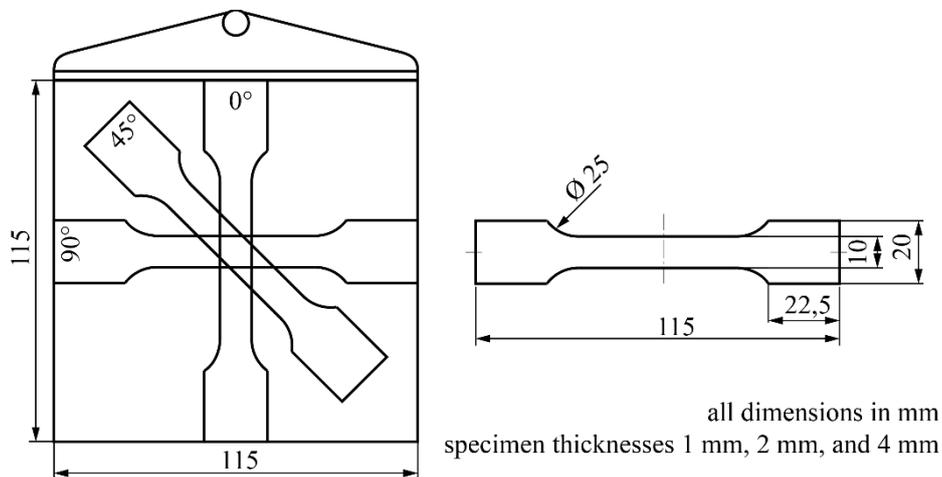
Figure 3: test specimens used for mechanical analysis and the different mold directions
