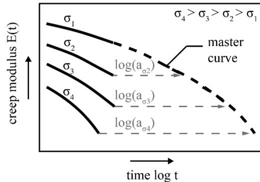
Figure 2: time stress superposition – schematically
