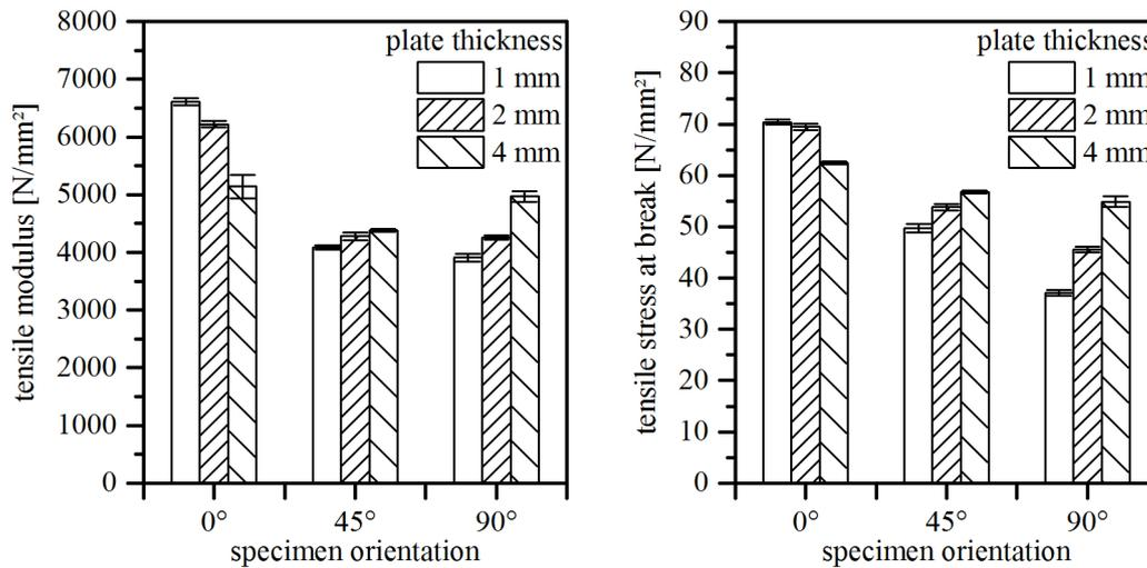
Figure 5: tensile modulus (left) and tensile stress (right) in dependence of the plate thickness and specimen orientation
