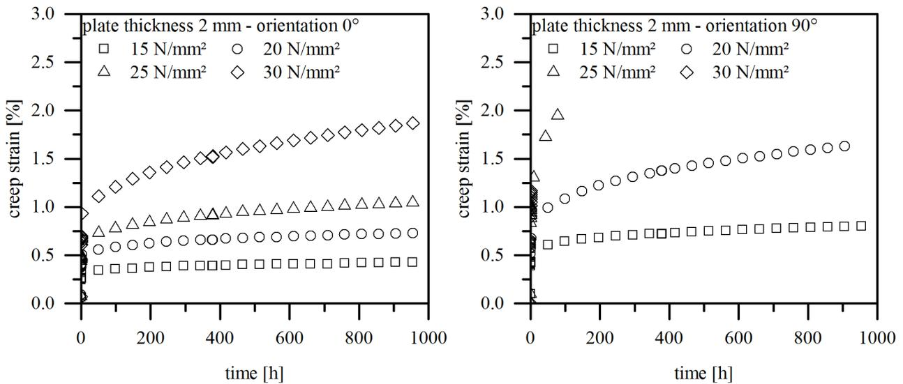
Figure 7: creep strain of test specimens with 2 mm thickness into flow direction  $0^\circ$  (left) and perpendicular to flow direction  $90^\circ$  (right)
