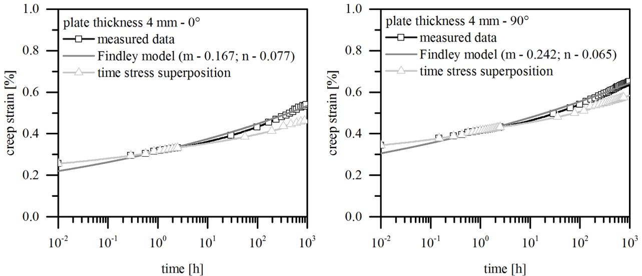
Figure 11: creep curves with experimental data, Findley model and time stress superposition for stress of 15 N/mm<sup>2</sup> and test specimen directions of 0° (left) and 90° (right)
