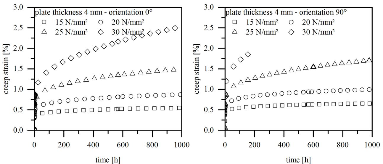
Figure 8: creep strain of test specimens with 4 mm thickness into flow direction  $0^\circ$  (left) and perpendicular to flow direction  $90^\circ$  (right)
