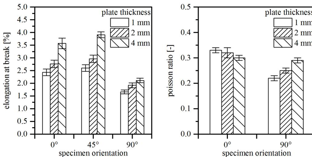
Figure 6: elongation at break (left) and Poisson's ratio (right)
