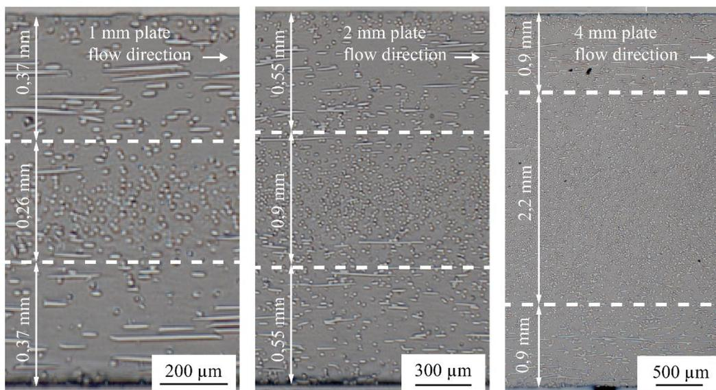
Figure 4: glass fiber orientation and layer formation in 1 mm, 2 mm and 4 mm sample
