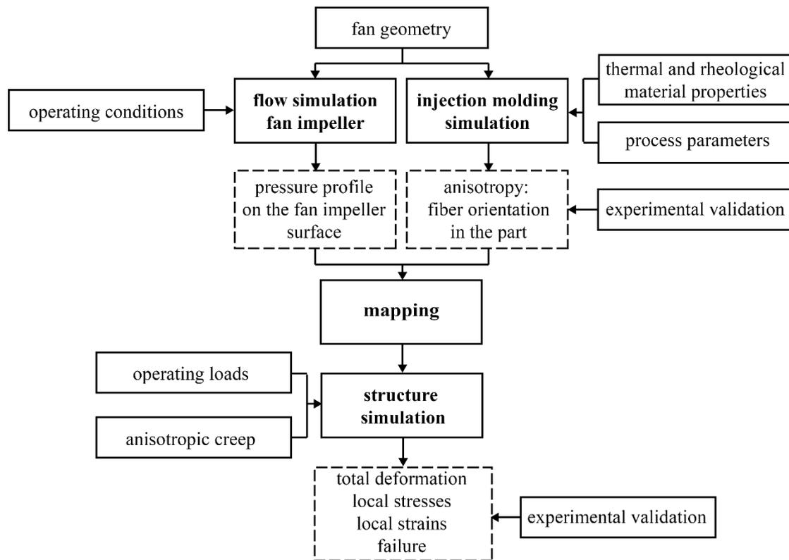
Figure 12: integrative approach to determine the time-dependent and anisotropic creep behavior of fan impellers
