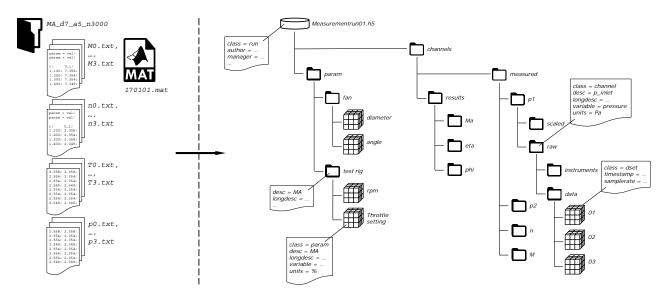
Figure 8: Comparison of the current data management approach based on directories and files to the proposed approach based on a modular data model and the HDF5 file format.
