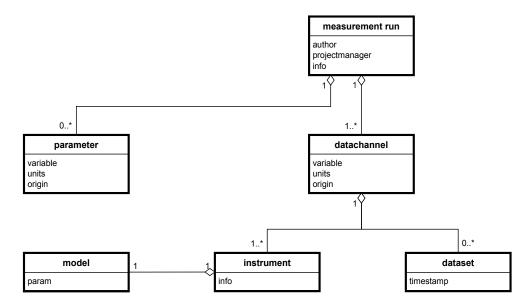
Figure 4: UML diagram showing the data model, forming a hierarchic structure of generic classes.
