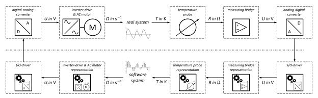
Figure 2: Exemplary arrangement of instrumentation for controlling the rotation frequency of an AC motor (left-hand side) and measuring a temperature (right-hand side).
