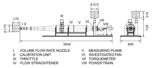
Figure 7: DIN 24163 compliant fan test rig utilized at TU Darmstadt for validation of efficiency scaling methods.
