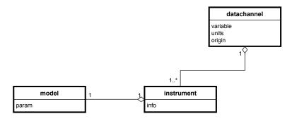
Figure 3: UML diagram showing the relationship of the introduced classes datachannel, instrument and model.
