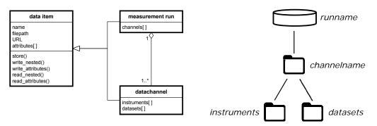
Figure 5: relation of the data item abstract class to generic data model classes (left-hand side) mapping of objects to the HDF5 file structure (right-hand side)
