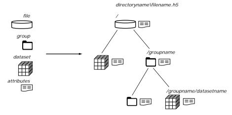
Figure 1: Overview of HDF5 base model objects and exemplary hierarchic data structure.
