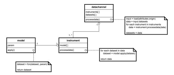
Figure 6: Mechanisms for automatic data processing with respect to corresponding instruments calibration.
