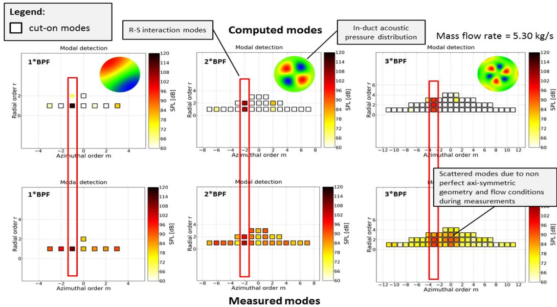
Figure 7: modal decomposition inside the fan duct (tonal noise)
