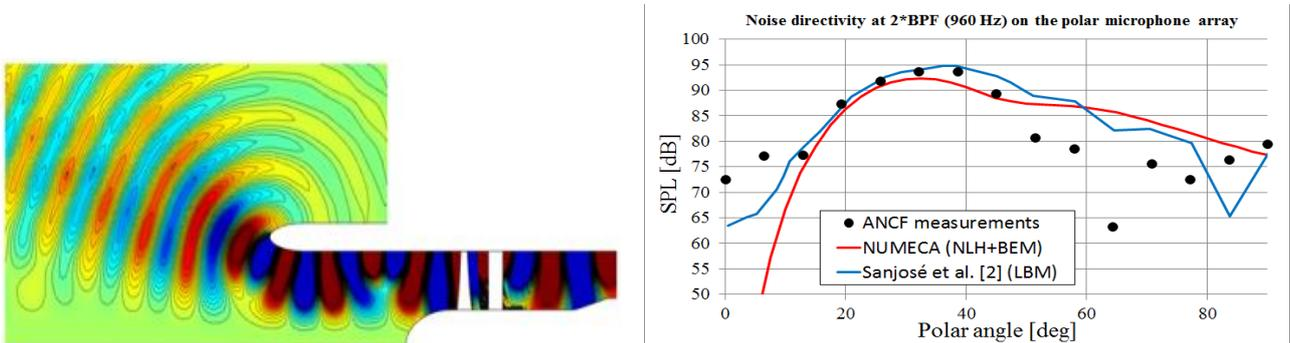
Figure 14: acoustic pressure field [Pa] and noise directivity plots at 2\*BPF (tonal noise)
