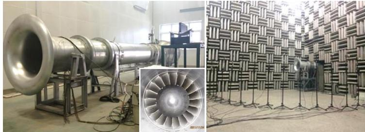
Figure 1: NPU fan rig tested in the semi-anechoic chamber
