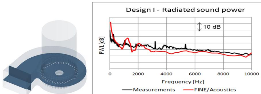
Figure 17: centrifugal compressor design I (size = 10x10x3.5 cm, RPM=8000, blades number = 40)
