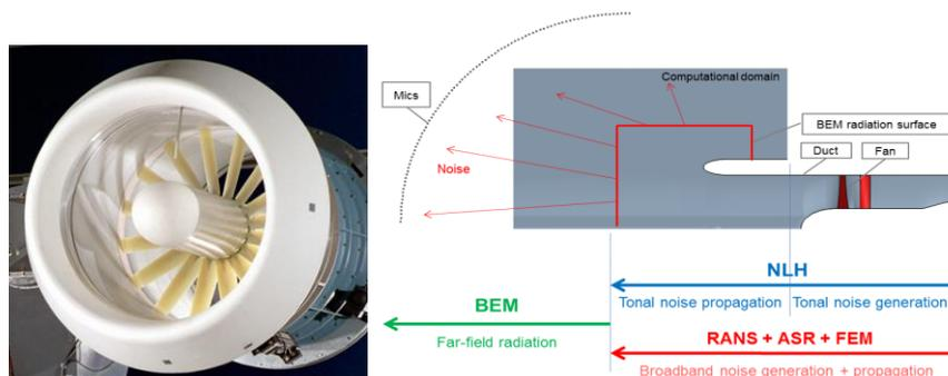
Figure 12: ANCF fan geometry (left) and relative computational domain (right)
