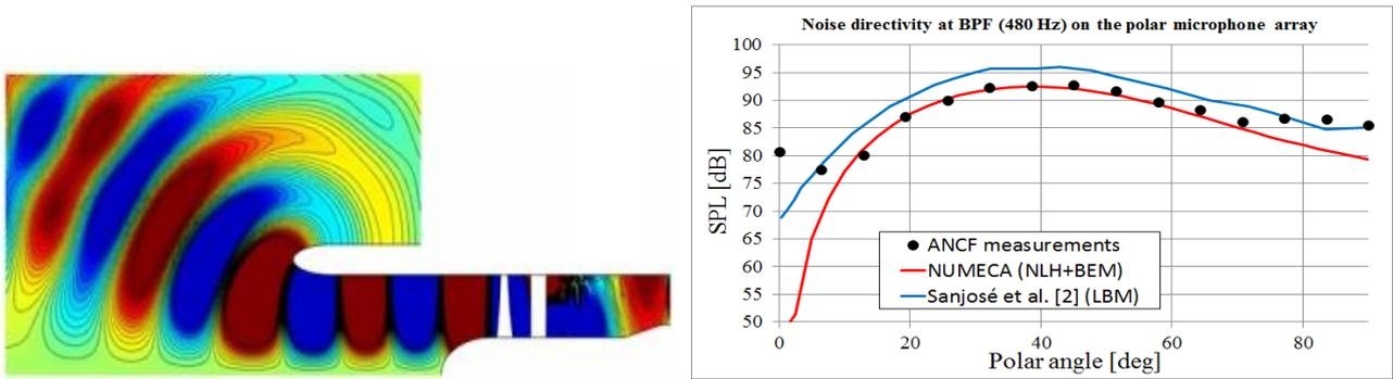
Figure 13: acoustic pressure field [Pa] and noise directivity plots at 1\*BPF (tonal noise)
