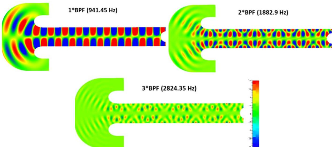
Figure 6: acoustic pressure field [Pa] inside the fan duct and in the near-field (tonal noise)
