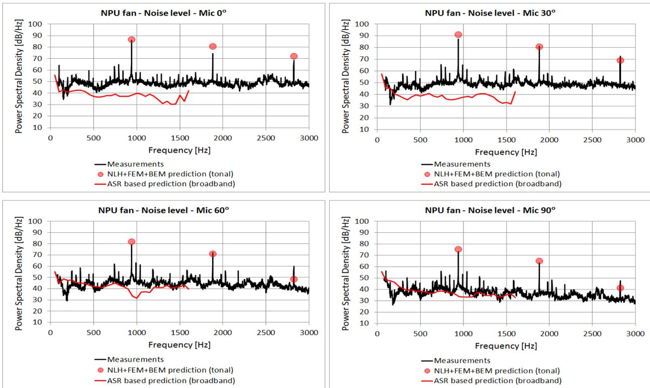
Figure 11: broadband noise spectra relative to different far-field microphones
