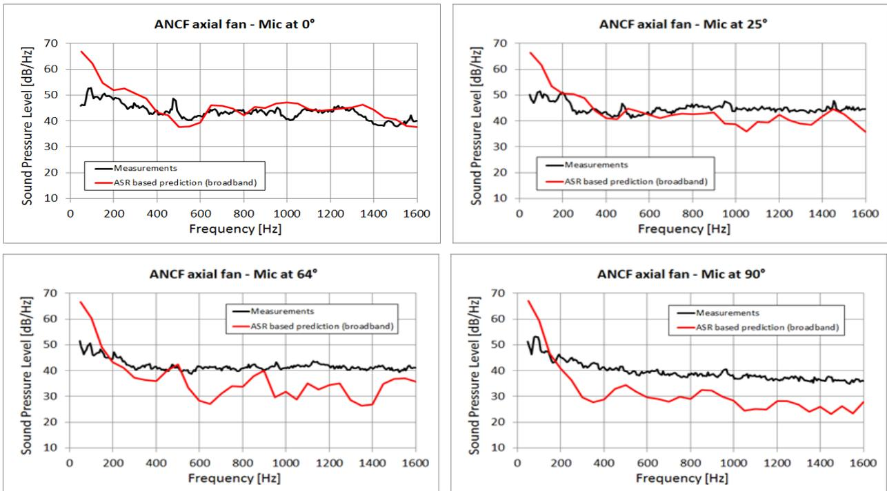
Figure 16: broadband noise spectra relative to different far-field microphones
