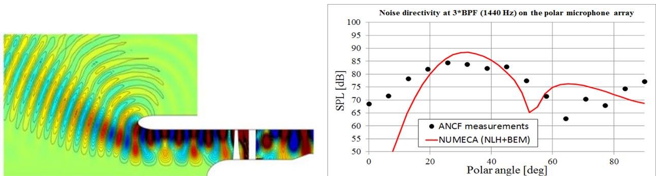
Figure 15: acoustic pressure field [Pa] and noise directivity plots at 3\*BPF (tonal noise)
