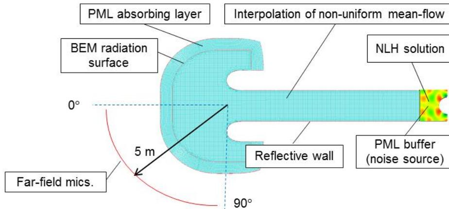
Figure 5: FEM-BEM computational domain and boundary conditions (acoustic mesh shown in blue)
