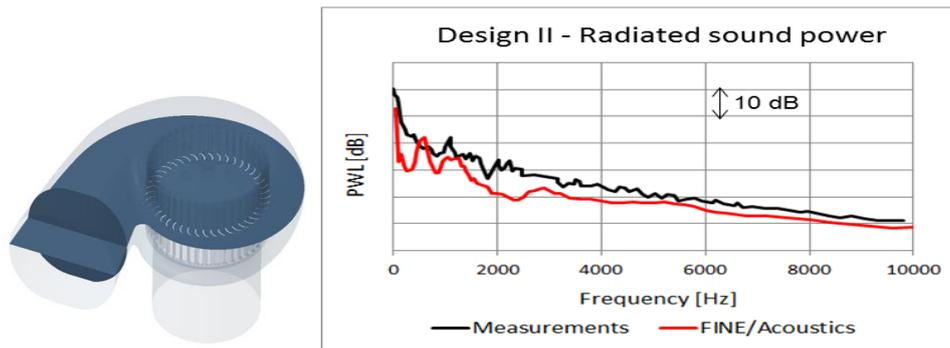
Figure 18: centrifugal compressor design II (size = 21x21x8 cm, RPM=3000, blades number = 44)
