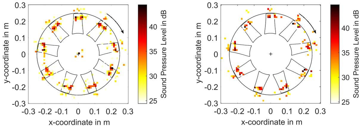
Figure 8: Beamforming map of the fan NIUG evaluated with the virtual rotating array method (left) and the modal decomposition method (right) for the third octave band with center frequency 5000 Hz
