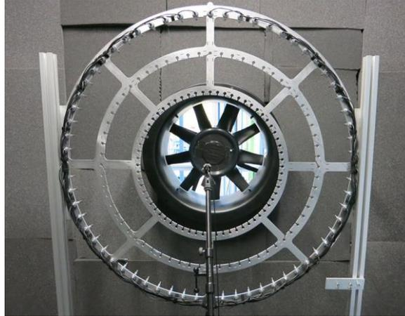
Figure 6: Generic test fan (rotational direction: clockwise) and microphone array
