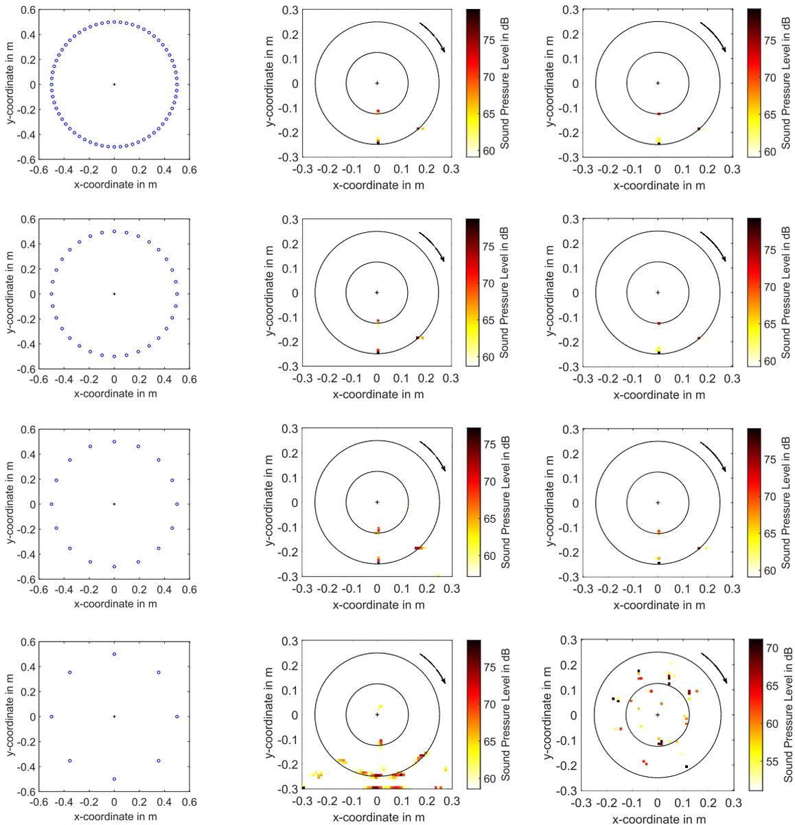
Figure 4: Position of microphones (left), beamforming map with virtual rotating array method (middle) and with modal decomposition method (right) for the third octave band with center frequency 2000 Hz
