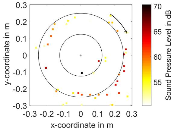
Figure 2: Smeared sound source distribution for  $n = \text{constant}$  for the third octave band with center frequency 2000 Hz
