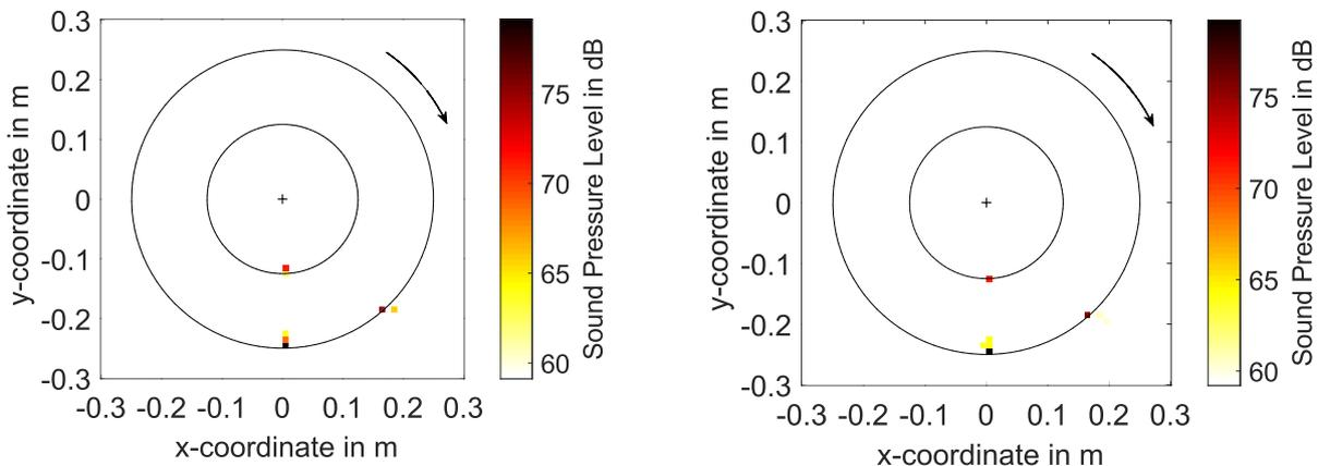
Figure 3: Correct focusing of the sound sources evaluated with the virtual rotating array method (left) and the modal decomposition method (right) for the third octave band with center frequency 2000 Hz
