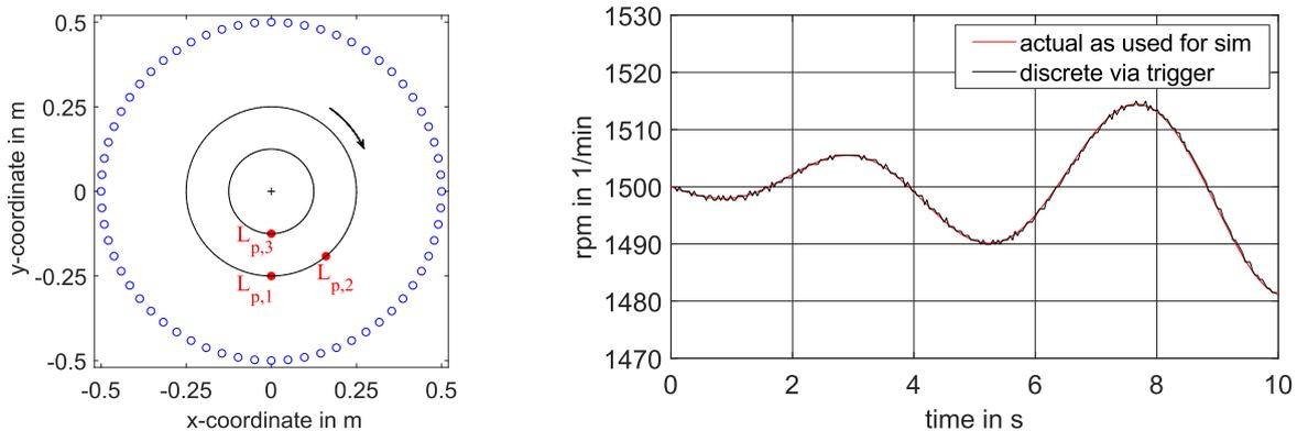
Figure 1: Left: Triggered position of the three sources (red markers), positions of the 64 microphones (blue markers). Right: Non-constant rotational velocity.
