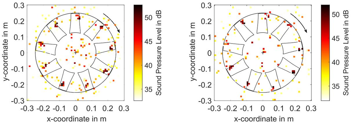
Figure 7: Beamforming map of the fan NIUG evaluated with the virtual rotating array method (left) and the modal decomposition method (right) for the third octave band with center frequency 2000 Hz
