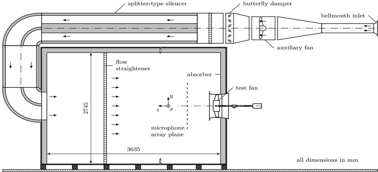
Figure 5: Standardized inlet test chamber according to ISO 5801
