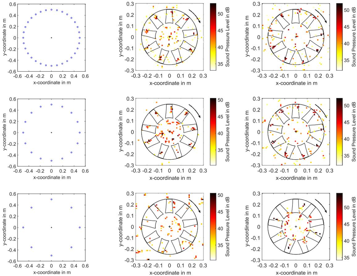
Figure A: Microphone positions (left), beamforming map with the virtual rotating array method (middle) and with the modal decomposition method (right) for the third octave band with center frequency 2000 Hz
