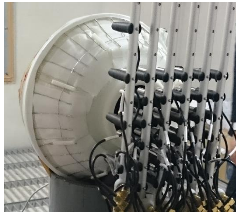
Figure5: Photograph of microphone array arrangement in front of the fan.
