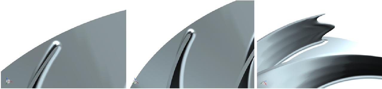
Figure 2: Illustration of the three trailing edge geometries, (left) thin straight, (middle) thick straight and (right) wavy.
