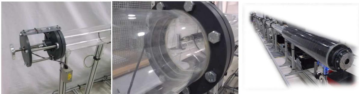
Figure 8: Aeroacoustic set-up with (left) the outlet throttle, (middle) a microphone with its nose cone and (right) the full device with the orifice plate and one anechoic termination at the foreground.
