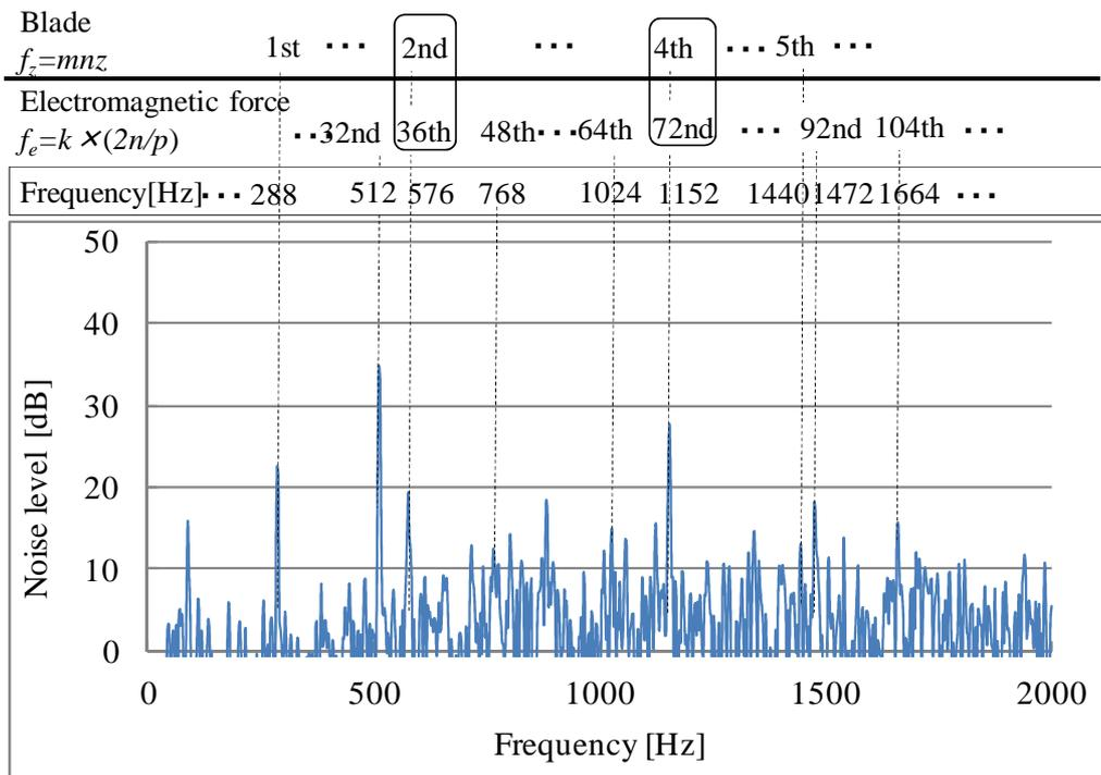
Figure 8: Noise level measured at 1922 min<sup>-1</sup>
