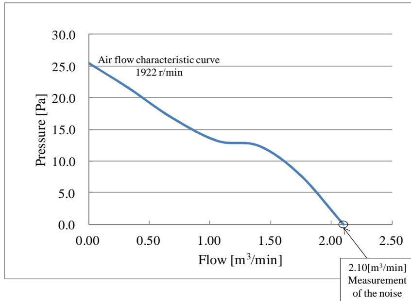
Figure 1: Air flow characteristic curve of the fan motor
