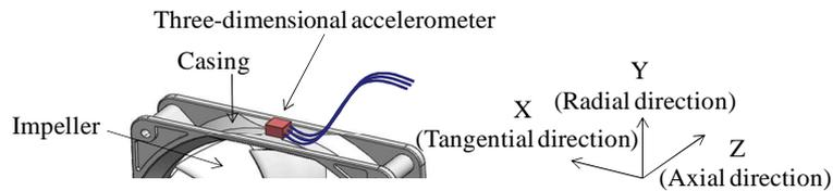
Figure 3: Measurements of measuring three-dimensional acceleration
