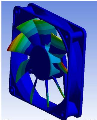
Figure 14: Natural frequency mode at 538 Hz by simulation
