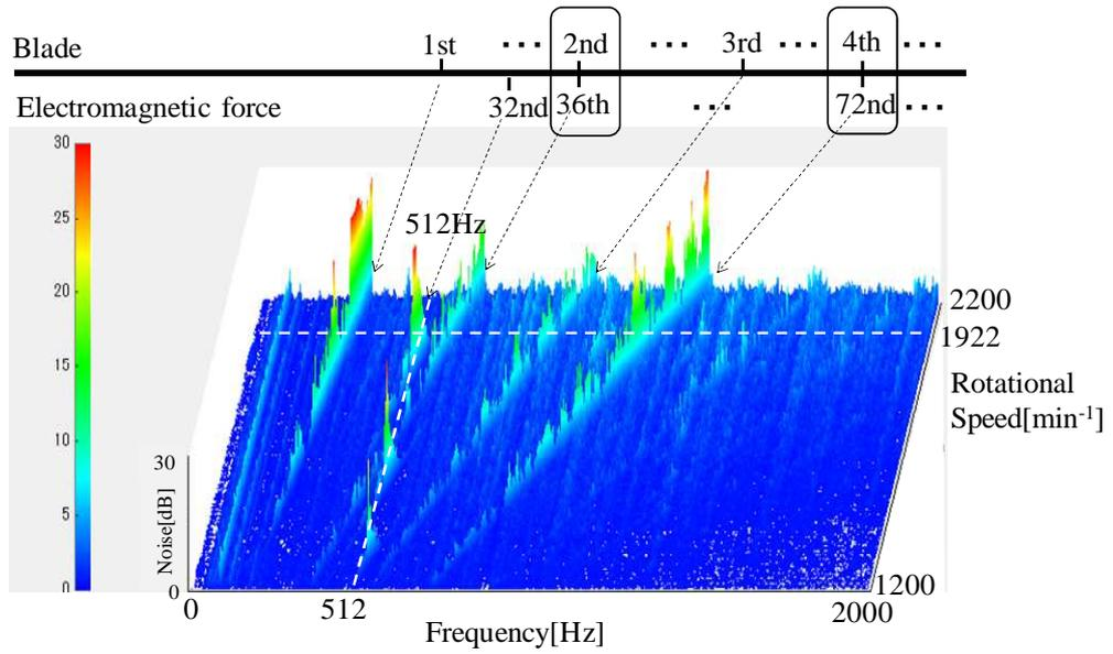
Figure 7: Natural vibration mode of the fan motor at 530 Hz
