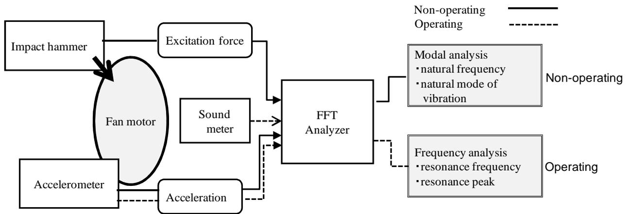
Figure 2: Block diagram of measurement system
