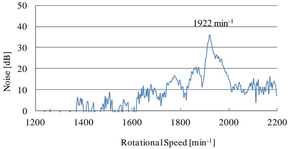
Figure 9: Noise level of the 32<sup>nd</sup> electromagnetic force
