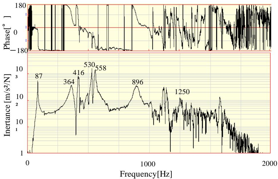
Figure 4: The Transfer function in the axial direction
