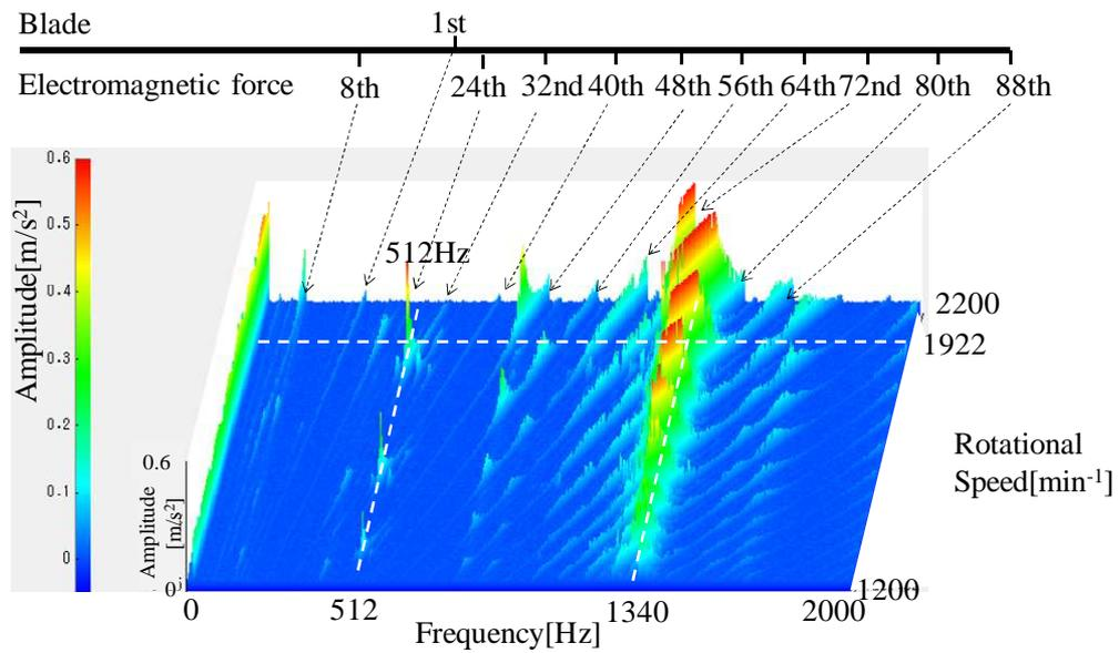
Figure 10: Vibration amplitude in the axial direction
