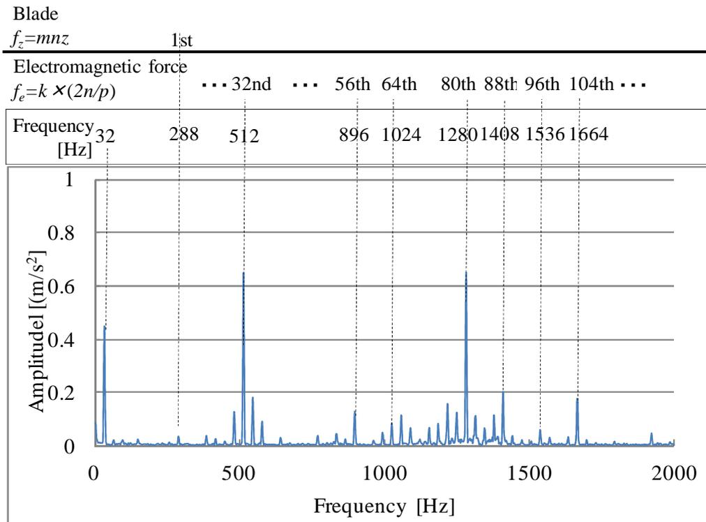
Figure 11: Vibration amplitude in the axial direction at 1922 min<sup>-1</sup>
