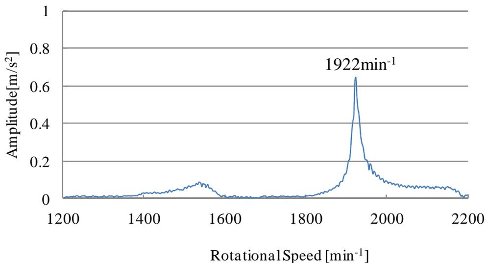
Figure 12: Vibration amplitude of the 32<sup>nd</sup> electromagnetic force in the axial direction
