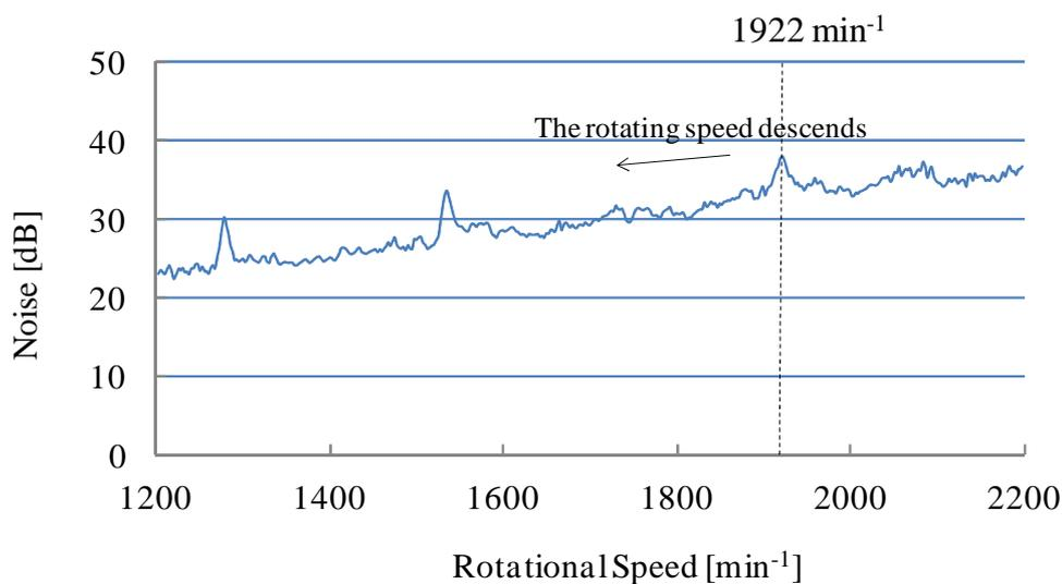
Figure 6: Overall noise level versus rotational speed
