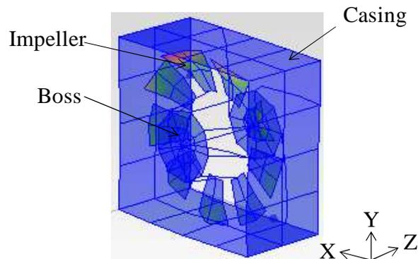
Figure 5: Natural vibration mode of the fan motor at 530 Hz
