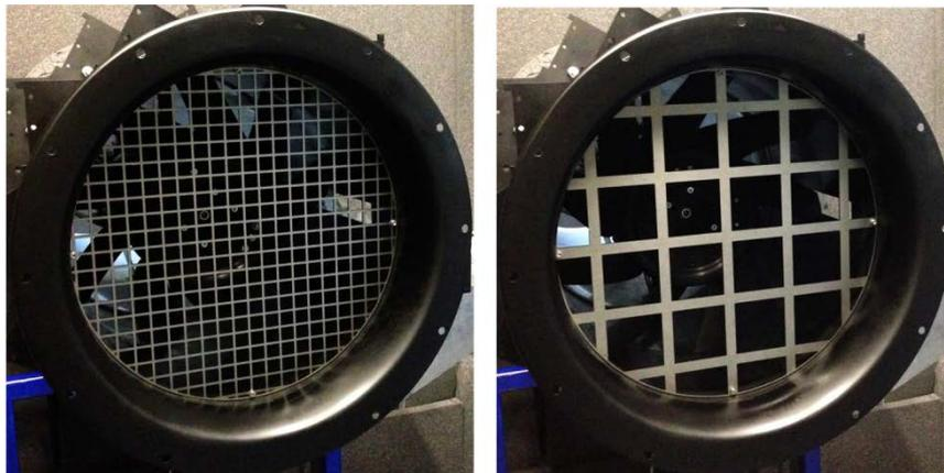
Figure 2: Turbulence grids - grid 20 (left) and grid 80 (right)
