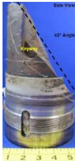
Figure 8 – Motor Shaft Failure
