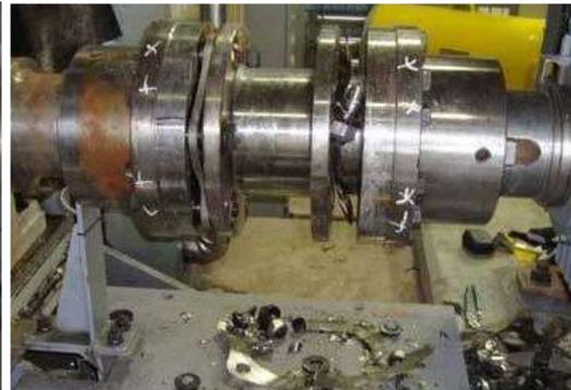
Figure 5 – Failed Disc Pack Coupling
