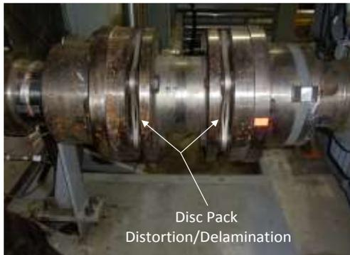
Figure 4 – Coupling Disc Pack Distortion
