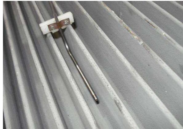
b: air velocity measurement (dynamic pressure) with Pitot tube
