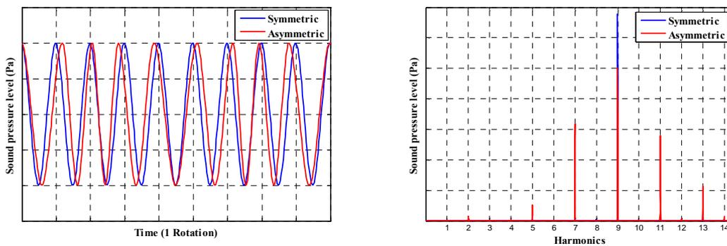
Figure 5: Blade passing induced signal in (a) time domain and (b) frequency domain for a 9 bladed design.
