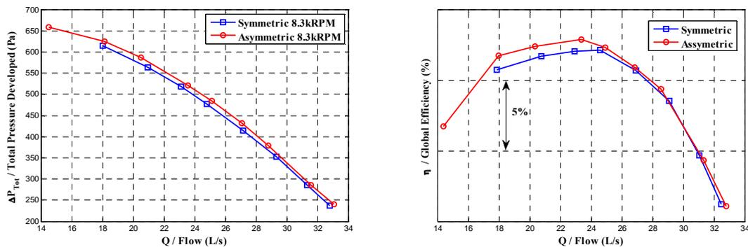
Figure 6: (a) Performance curves and (b) efficiency curves of compressors
