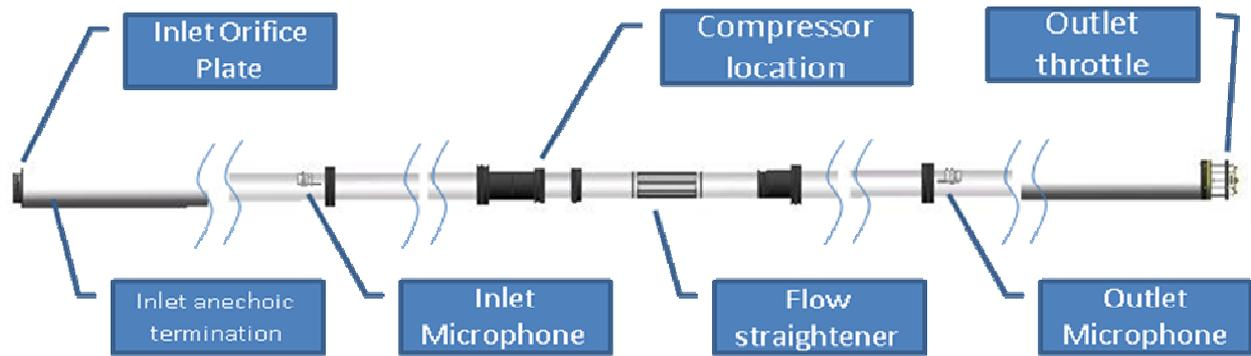
Figure 2: Aero-acoustic set-up
