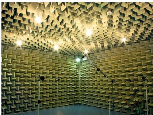
Figure 3: (a) Semi-anechoic chamber
