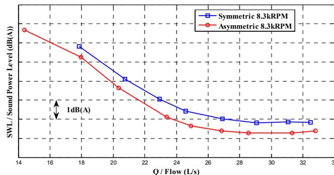
Figure 7: Sound power level of compressors
