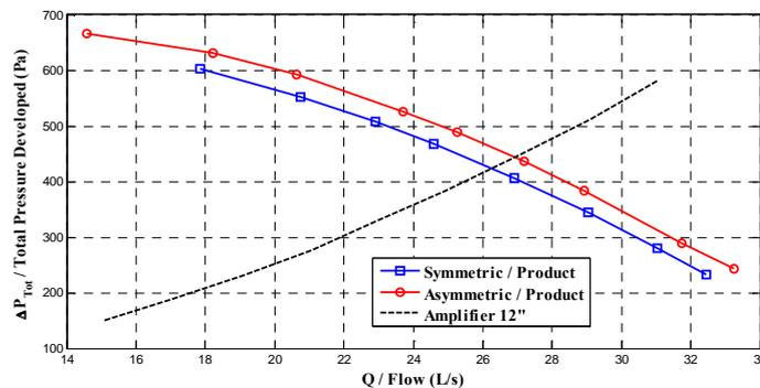
Figure 9: In product performance curve and restriction curve of the amplifier
